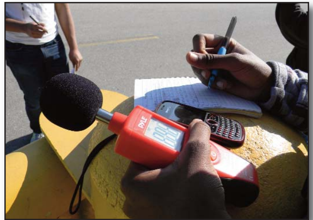
Using a sound level meter to measure noise at Baldwin Hills Scenic Overlook State Park
